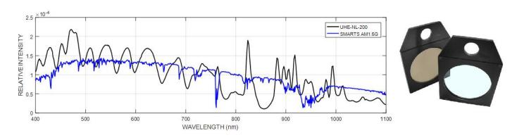
UHE-NL with AM1.5G-FT-3 filter installed providing class A spectral match to the AM1.5G spectrum
