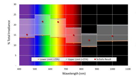
15.1774% 400-500 Class A nm = 500-600 21.5593% Class A nm = 600-700 21.3764% Class A nm = 700-800 nm = 14.9445% Class A 800-900 nm = 12.4609% Class A 900-1100 nm = 14.4815% Class A
